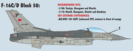
Turkish Air Force F-16C/D Block 50 aircraft are externally very similar to USAF F-16CJ. These aircraft were not equipped with the parabrake housing, and have no external ECM antenna either. The only major visual difference is the advanced AIFF antenna ("bird slicers")(1) in front
