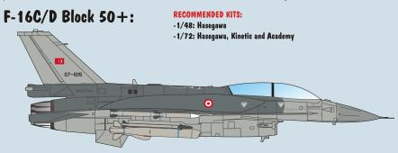
At the time that these decals were designed (August 2011), the only Turkish F-16C/D Block 50+ delivered was 07-1015, which was equipped with low-profile (CCIP-type) AIFF antenna, an avionic spine and CFTs and looked largely similar to aircraft delivered to Singapore, Poland and Greece earlier. We expect the single-seater Block 50+ to look similar; with a parabrake housing, enlarged nav lights, ECM antenna and low profile AIFF antenna.
